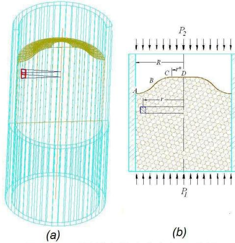
Fig. 2. The front shape of grease volume in pipe
